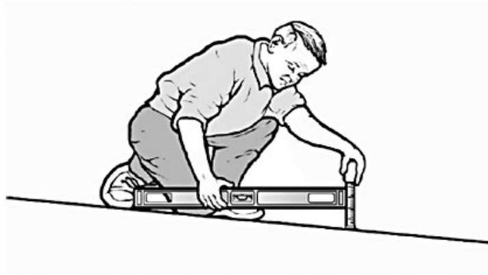
Measuring slope using a 24 inch bubble level and tape measure
